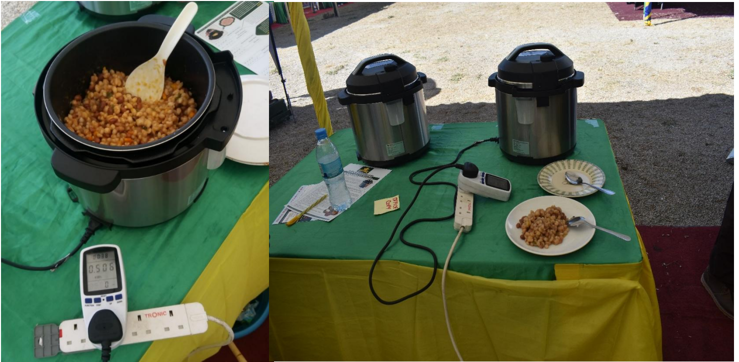
0.506 kilowatt hours (kWh) used to cook ¾kg of pounded maize with beans
