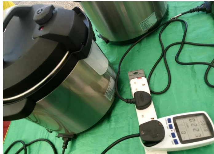
0.227 kilowatt hours (kWh) was used to cook \frac{3}{4} kg of rice
